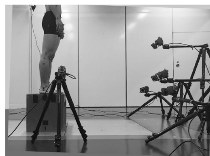
Fig. 1 Measurement setting. To focus on the foot, six of the 17 cameras used for measurement were placed around the feet
